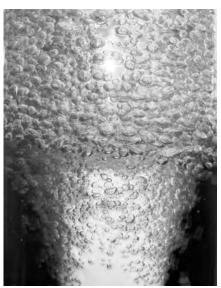
Bubbles with Monoflex 40 Micron Sparge Point
