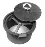
allow replacement of the Buna-N seal without the use of glue. A removable brass label plate is attached to the rim to allow for stamping of the well number. Morrison manholes have been independently tested to meet AASHTO standard for "H-20" truck loadings, ASTM A48, and section 206-3 of the American Public Works Association. Each 519 series manhole is individually boxed and supplied with a wrench.
