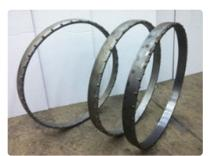
24-inch x Heavy Duty x Button Style Ring-Bit pictured with new induction braising process
