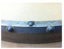
Button (Dome) style carbide insert bit highlighting our induction braising process.
