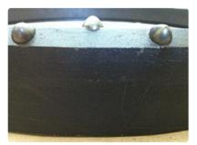
New Conical (Ballistic Carbide) insert bit, prior to our induction braising process.
