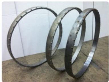
24-inch x Heavy Duty x Button Style Ring-Bit pictured with new induction braising process
