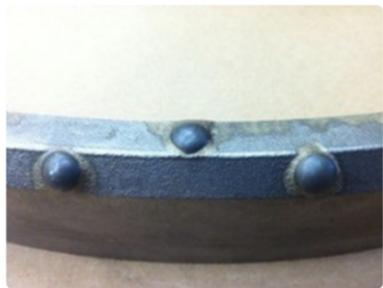
Button (Dome) style carbide insert bit highlighting our induction braising process.
