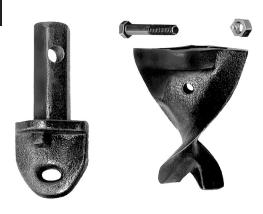
Especially designed cast steel bit eliminates "dead-spot" at hole center and bores clean, straight holes through semi-consolidated clay, loam, sand, gravel and similar formations. Cutterhead part number includes bit and shank complete. Bolt and nut included in assembly. Sizes are identified by the hole size, not actual flight diameter.
