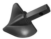
The STINGER's self-centering one-piece, cast steel construction with a smooth contoured shape permits free flow of material to the auger flight. Interchangeable with the two-piece Fishtail bit, it works well in clay, loam, sand, gravel and similar formations. Designed for use with standard construction and  $\mathbf{HEX-COR}^{\mathsf{TM}}$  augers and as a pilot bit with large diameter hollow stem augers. Sizes are identified by the hole size, not actual flight diameter.
