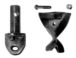
Especially designed cast steel bit eliminates "dead-spot" at hole central and bores clean, straight holes through semi-consolidated clay, loam, sand, gravel and similar formations. Cutterhead part number includes bit and shank complete. Bolt and nut included in assembly. Sizes are identified by the hole size, not actual flight diameter.
