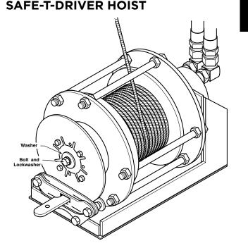
The SAFE-T-DRIVER® hoist is a hydraulic hoist which is designed to replace the cathead for SPT sampling operations. Unlike the cathead, SAFE-T-DRIVER hoist offers full safety of operation and requires very little physical exertion to operate. The SAFE-T-DRIVER hoist is operated by a valve lever which is used to **control the lift** and free fall the hammer for each blow. The hoist can be used to "bump out" the loaded sampler at the end of a run.
