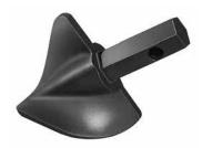
The STINGER's self-centering one-piece, cast steel construction with a smooth contoured shape permits free flow of material to the auger flight. Interchangeable with the two-piece Fishtail bit, it works well in clay, loam, sand, gravel and similar formations. Designed for use with standard construction and  $\mathbf{HEX-COR}^{\mathsf{TM}}$  augers and as a pilot bit with large diameter hollow stem augers. Sizes are identified by the hole size, not actual flight diameter.
