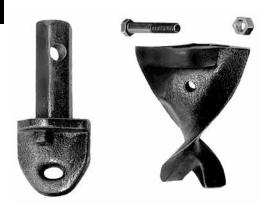
Especially designed cast steel bit eliminates "dead-spot" at hole center and bores clean, straight holes through semi-consolidated clay, loam, sand, gravel and similar formations. Cutterhead part number includes bit and shank complete. Bolt and nut included in assembly. Sizes are identified by the hole size, not actual flight diameter.
