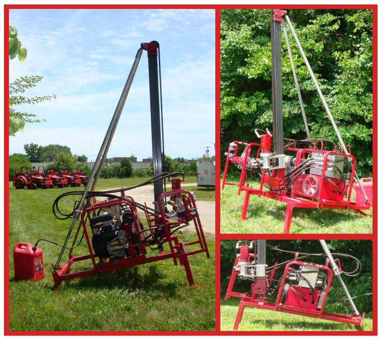
The V2000 is a people-portable and heliportable, hydraulic powered drill designed for geotechnical and seismic exploration. With 2 mast stabilizers for more rigid mast positioning, the V2000 is a tough, high performance drill with go-anywhere versatility.
